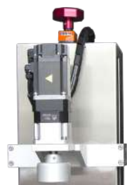
鎖蓋裝置 (伺服驅動) Capping system (Driven by servomotor)
