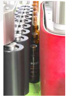
連動式扶瓶機構 Interlocking bottle clamp
