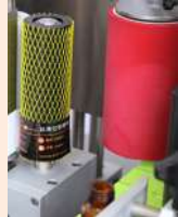
預先剔除標籤滾輪 Pre-rejection roller for defective label
