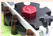
星盤式分瓶裝置 Indexing bottle separation device
