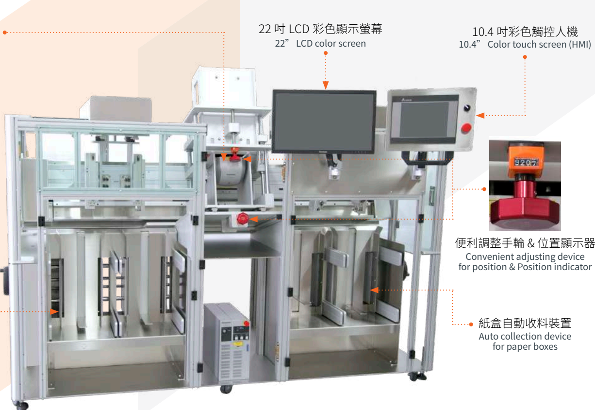
Panasonic 雷雕主機 (日本製) Panasonic laser marking machine (Made in Japan)
